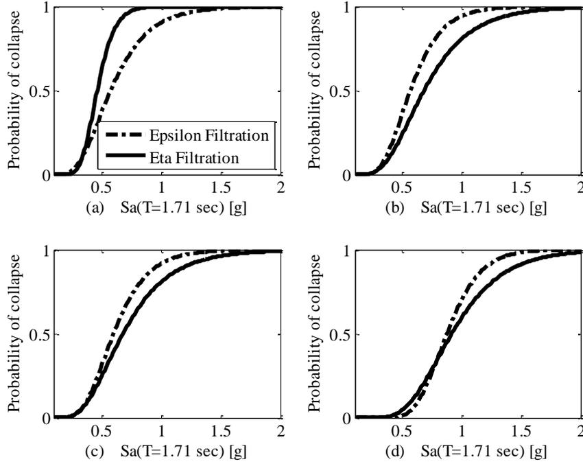
Figure 10: Fragility curves in four different hazard levels for two Epsilon and Eta filtration approaches; (a) 200 years; (b) 400 years; (c) 475 years; (d) 2475 years.
