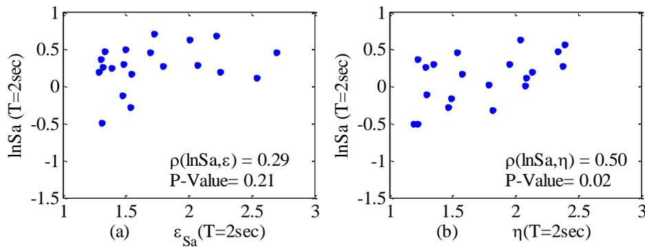
Figure 4: Correlation between collapse pseudo acceleration of MDOF structure (ID 1019) for 20 filtered records with (a) in the case of Epsilon, (b) in the case of Eta.
