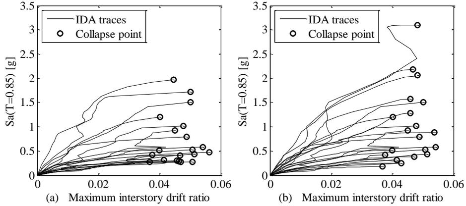
Figure 15: The IDA curves for SPEAR building; (a) based on twenty records which are compatible with CMS; (a) based on 20 records which are compatible with E-CMS.
