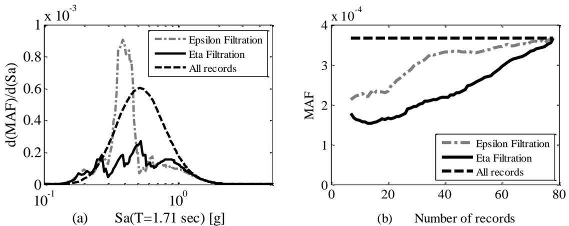
Figure 11: (a) The MAF for the considered eight story structure (ID 1011) with  $T=1.71$ s; (b) The MAF variation versus number of employed records for building ID 1011.
