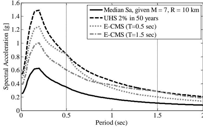
Figure 8: Eta-based conditional mean spectra in different periods for an equal probability of exceedance 2% in 50 years. ( $T^*=0.5$  sec &  $T^*=1.5$  sec).
