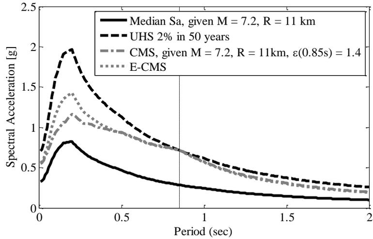
Figure 12: UHS, CMS, E-CMS and the median spectra for the assumed site of SPEAR building which is the same as Figure (6).
