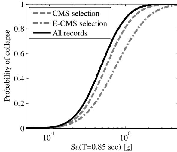
Figure 16: The fragility curves for SPEAR building in 2475 years hazard level.
