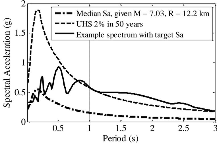
Figure 1: Median predicted spectrum, UHS for 2 % probability of exceedance in 50 years and the example spectrum which is the Newhall-W Pico Canyon Rd with  $M=6.7$  recorded from Northridge event [18].
