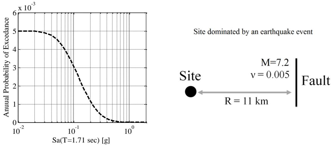
Figure 9: (left) the seismic hazard curve for the given scenario; (right) a schematic representation of the chosen seismic scenario.
