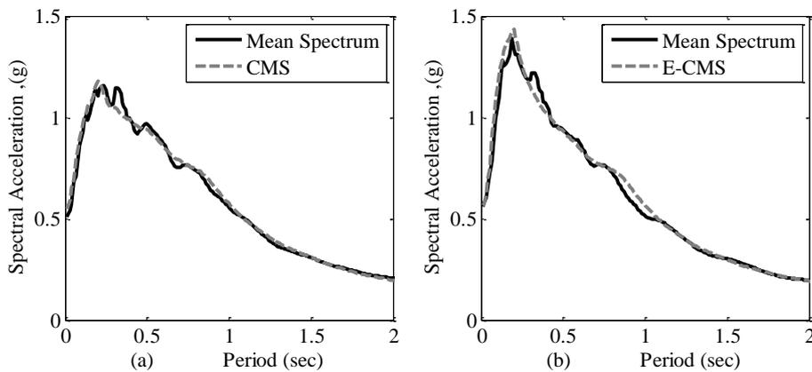
Figure 14: (a) The mean spectrum of 20 selected records and the CMS; (b) The mean spectrum of 20 selected records and the E-CMS.
