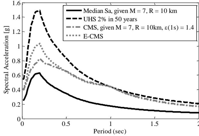
Figure 6: UHS, Epsilon-based and Eta-based conditional mean spectrum for an ideal site, given  $M=7$ ,  $R=10$  km,  $\epsilon=1.4$ .
