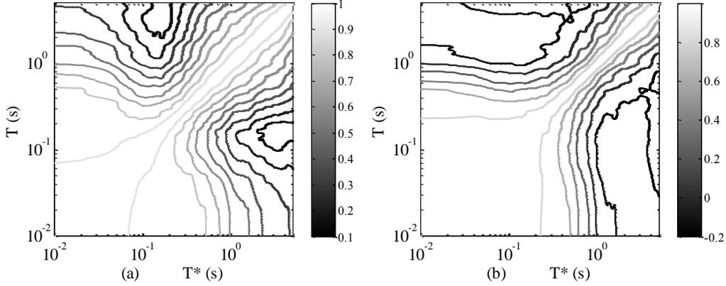
Figure 5: Empirical correlation coefficients based on the considered GMR database. (a) For Epsilon. (b) For Eta. ( $T$ : Period of interest,  $T^*$ : Target period)
