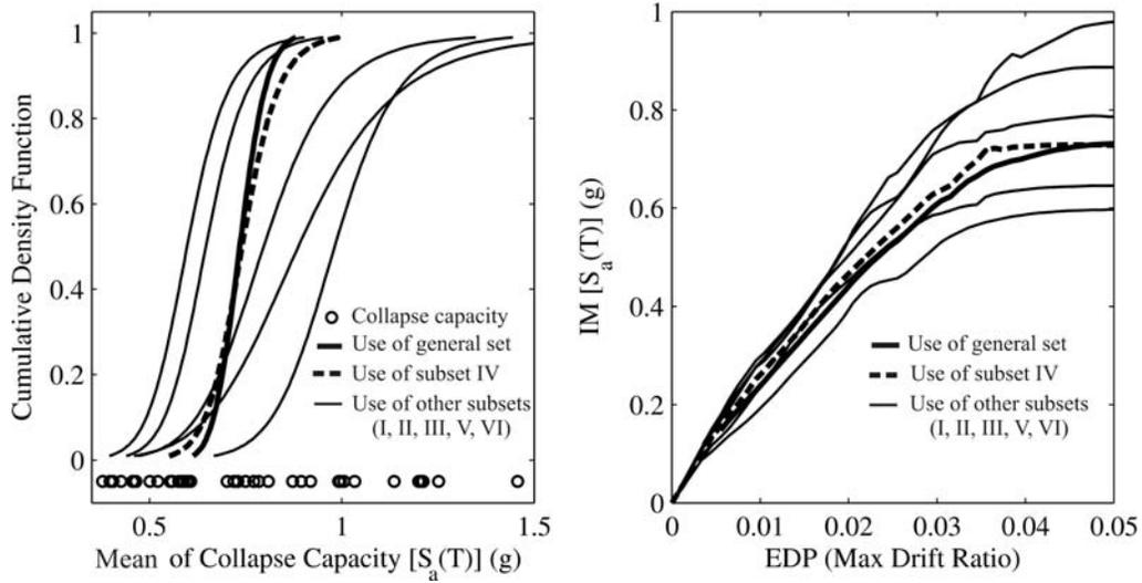
Figure 6. Efficiency assessment of the proposed subsets: (a) The CDF of the mean value of the seismic collapse capacity, (b) the mean of the full IDA analysis using different proposed subsets and the general set.
