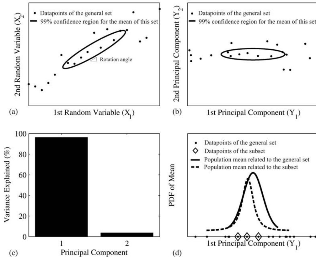
Figure 4. The Role of PC analysis in reduction of subset size: (a) a high correlation between the two variables can be observed, (b) the transformed data confirm the independency of the PC's, (c) the first PC contains 95% of the required information, and (d) there is good agreement between the probability density functions corresponding to the general and the subset.
