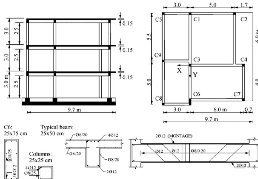
Figure 5. The elevation (upper left) and plan (upper right) view of the test-structure, showing typical reinforcement details (bottom).
